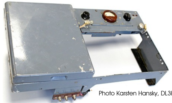
The metal frame in which the receiver was mounted. Note the three sockets at the bottom to connect an external LT battery and an aerial.
