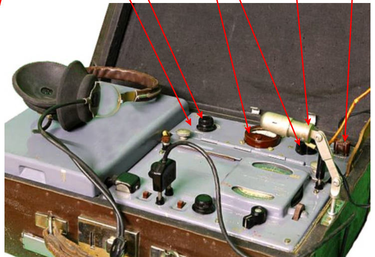
The suitcase was opened, revealing the battery/accessories compartment on the left, the PR-56A receiver at the bottom right, and a panel with filament voltage adjustment, meter, meter switch, and operator lamp socket.
