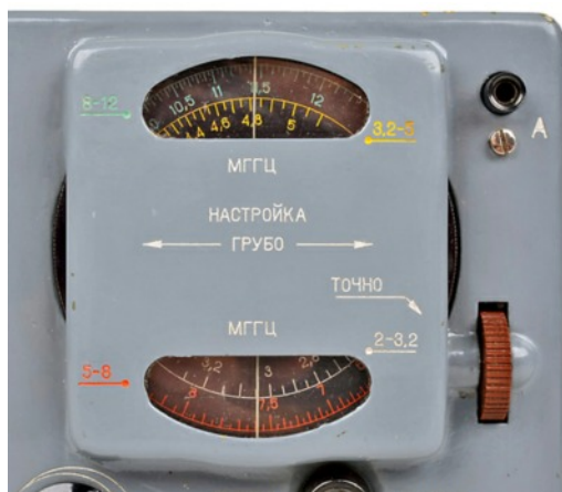
Detail view of frequency scales and tuning arrangements. Course tuning was done with the large black frequency scale which extends at both sides. The brown thumb wheel at the right was used for fine-tuning.
